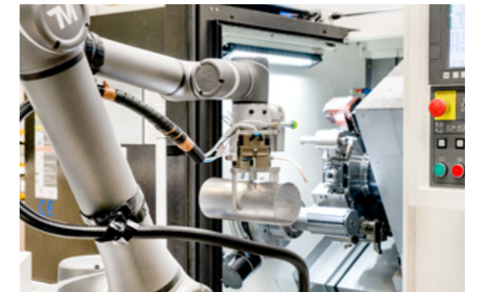
Turn-mill centre with collaborative robot
