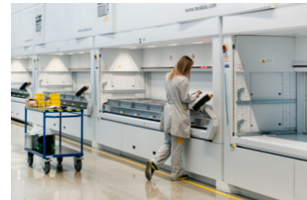
Automated vertical storage system
