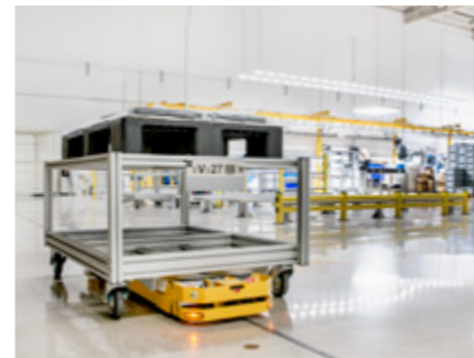
Automated guided vehicle for flexible internal logistics
