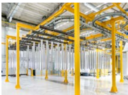
Modern powder coating system with low water and energy consumption, pre-treatment tunnel with passivation (corrosion protection), and automated powder application with a recovery system.
