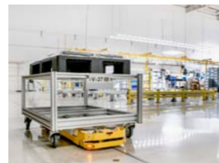
Automated guided vehicle for flexible internal logistics
